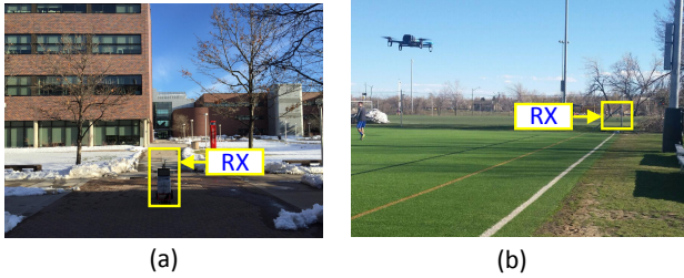
Figure 5: The setup to validate the effects of changing the environments: at our campus in a downtown city (a) and at an open field (b).
