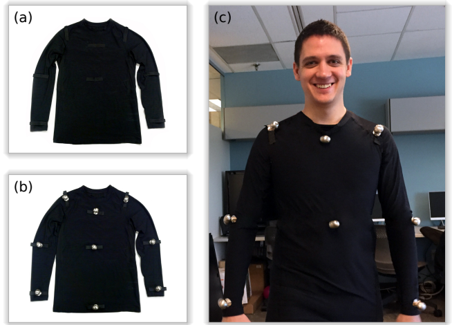
Fig. 7. Thermal posture ground-truth and training suit (a) with attachable metal spheres (b). The suit is worn during the training process to identify the relationship between the patient’s thermal volume and joint positions (c).
